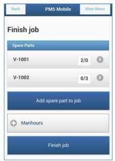
Once the consumption is saved, the application switches back to Finish Job screen for currently selected job. New consumption is now listed in spare part consumption list.
