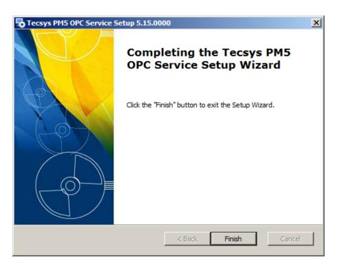
7. After installation, user can confirm that the PM5 OPC component is installed correctly and is running by opening Services list running on the computer and verifying that the service is present and running. Services list is easiest opened by typing *services.msc* in Run field of Windows.
