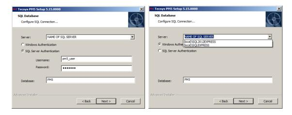
Once necessary data is entered, press button 'Next' to proceed. Installation package will now validate entered information (connection to SQL Server and provided user credentials) and if validation is successful, the installation of PM5 client will commence.
