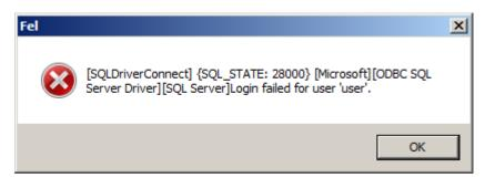
This error is shown when user specified for communication between installation package and SQL Server is invalid. When this error occurs, please double-check following:
