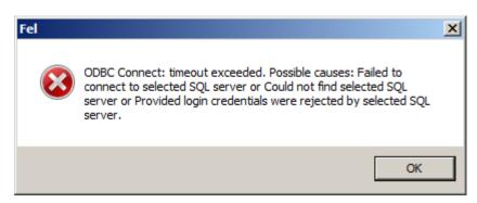
This error indicates that PM5 installation package could not find or was otherwise stopped from connecting to the SQL server specified by user. This issue is usually caused by:
