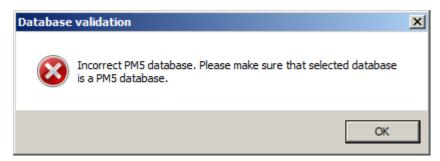
This error is shown when user runs an installation of PM5 client with pre-existing database and the selected database is not a PM5 database. To resolve this issue user needs to enter name of a valid PM5 database.
