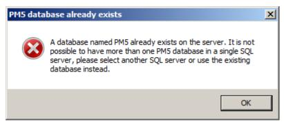
Error message above is shown if a database with name PM5 already exists on the SQL server that user is trying to use for the installation. Since two databases with same name cannot exist on same SQL server, user needs to either delete or rename the already existing database before an installation can be completed. Alternatively, user can select to use the already existing database for the installation.
