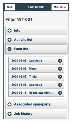
Fault list section shows all **unfinished** faults reported for currently selected machine. Every position in the list shows date on which the fault was reported and fault type.
