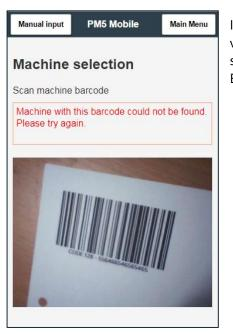
If scanned barcode is not found or PM5 is unable to handle scanned value, an a message or error text will be displayed on the screen for 5 seconds. Once it disappears, PM5 is ready for another barcode scan. Example of such scenario is shown in picture to the left.
